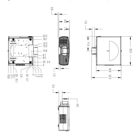
Figure 7-1. Vision 65/75 Dimensions (with Optional Fixed Anamorphic Lens)
